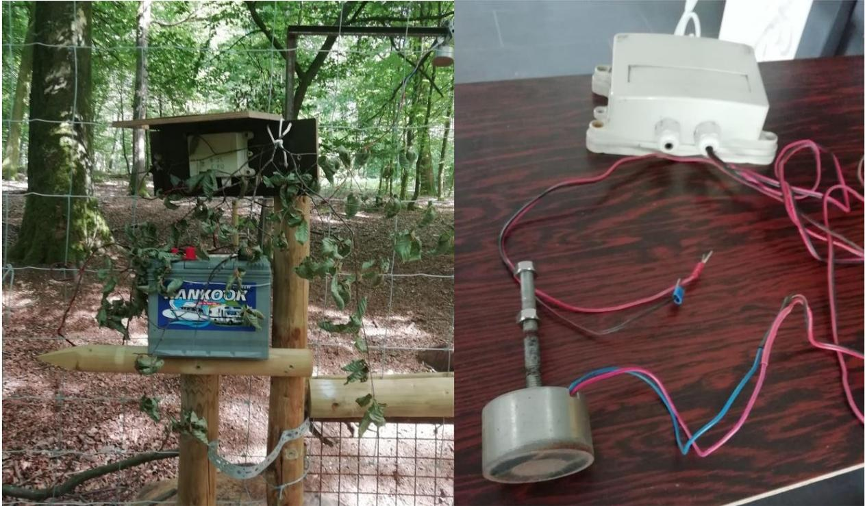
Figures 10 et 11 – Left: the remote triggering system installed in the field (battery, housing and magnet). Right: the box in charge of remotely breaking the current and thus the magnetic field of the magnet.
